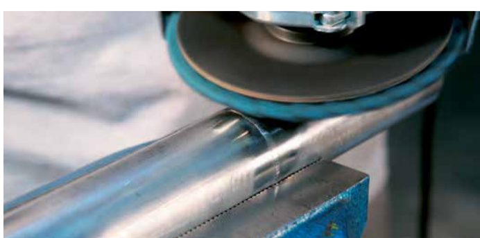
Post-processing of a welding seam using a polishing flap disc
