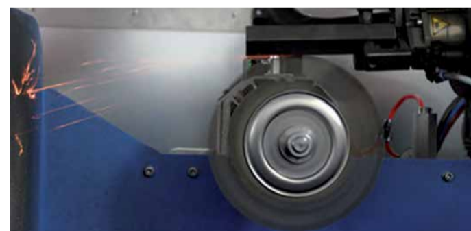
A brush (left) produces more than 95% fewer sparks than a grinding disc
