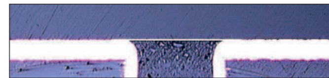
Cross-section of a bore of 0.50 mm – enlarged 100:1. Base copper only 18 µm. Deburred with LIPPROX® and perfectly metallized.
