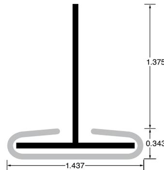
T-Shaped Holder (with PVC Seal) (BT90CS)
