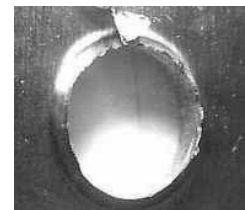
Class Five Extruded burrs are very large burrs that extrude from the base material. These burrs need to be preconditioned before brushing.
