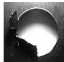
Class Four Well attached large burrs are large in nature and have a larger attachment point than a Class Three burr.
